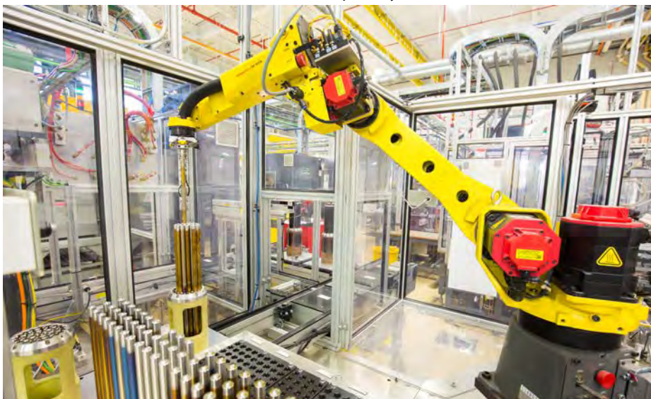
Figure 5 Cameco's Fuel Manufacturing Facility, Ontario, Canada (A state-of-the-art robotic arm assembles natural uranium fuel bundles)
