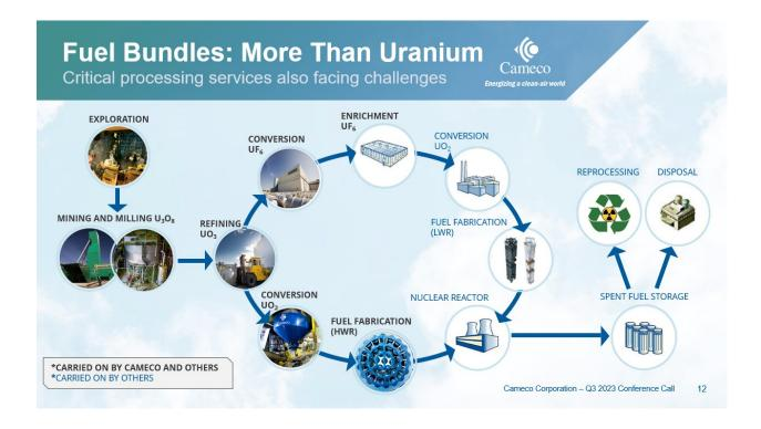
The services: refining, conversion, enrichment, de-conversion, pelletization, and fuel fabrication are getting more attention than ever, and the degree to which they are interdependent complicates the typical supply/demand analysis of a commodity. Those other segments of the fuel cycle are also facing challenges.
