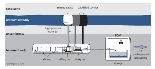
We have divided the orebody into production panels and at least three production panels need to be frozen at one time to achieve the full annual production rate of 18 million pounds. One JBS machine will be located below each frozen panel and the three JBS machines required are currently in operation. Two machines can be actively mining at any given time while the third is moving, setting up, or undergoing maintenance.
